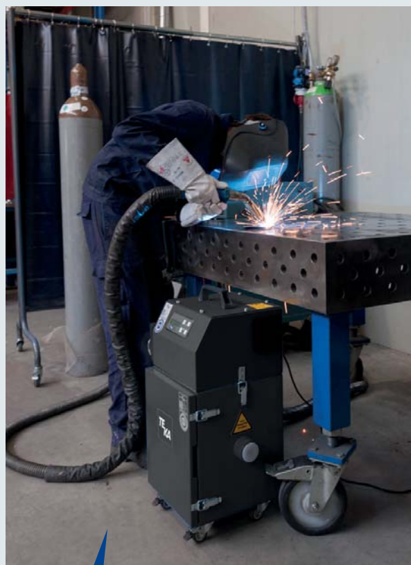
Example of application: Torch extraction
