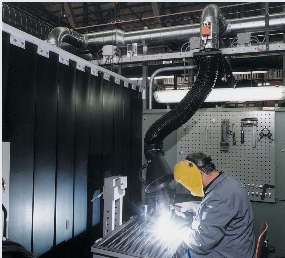
Example of application: Telescopic suction arm in a welding booth
